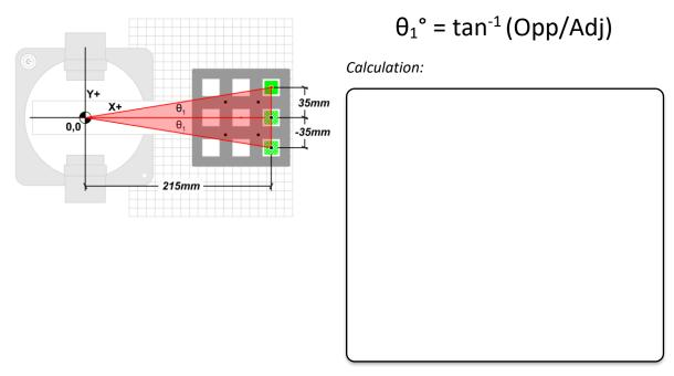
6. In the space provided above, calculate the correct roll angle for position 4. Show your work even though you are using a calculator.
