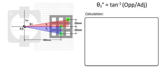
7. In the space provided above, calculate the correct roll angle for position 4. Show your work even though you are using a calculator.
