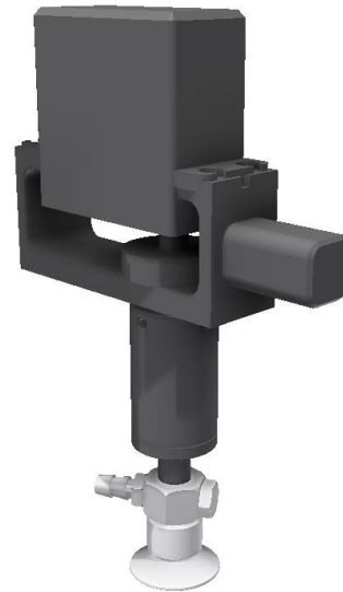
Suction cup gripper attached to the rotational servo.
