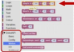
Adjust the X, Y, and Z movements as needed
