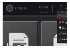
6. Now open the *Teach and Playback* module and perform a pick and place with a wooden cylinder as you did in a previous activity. The only difference is that this time you will use the Suction Cup to pick and place the object. Be sure to use "above" positions. Save your program when finished. You may even be able to use a program you have already written and just touch up the points.
