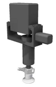
Suction cup gripper attached to the rotational servo.
