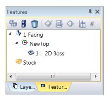
Use the feature finder to allow EdgeCAM to evaluate the 3D CAD model in order to break the model into manufacturable features
