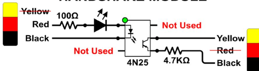
Connect EIO13 on the back of the robot to the input of the handshake controller, and then wire the output of the handshake controller to digital input #1 on the VEX Cortex. Use servo extensions to do this.
