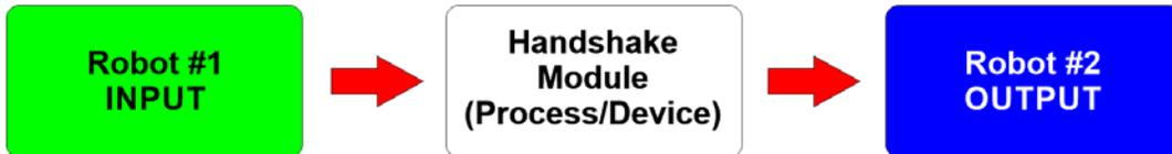
**Open Loop System Block Diagram:** Robot #1 acts as the input for robot #2. Robot #2 does not communicate back to robot #1 so there is no feedback. The Handshake Module acts as the device that helps make the handshake happen safely.
