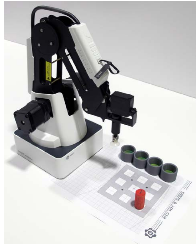
Dip Tank Set Up using 3D printed dip tanks and a Dobot field diagram. In this diagram four tanks are used.
